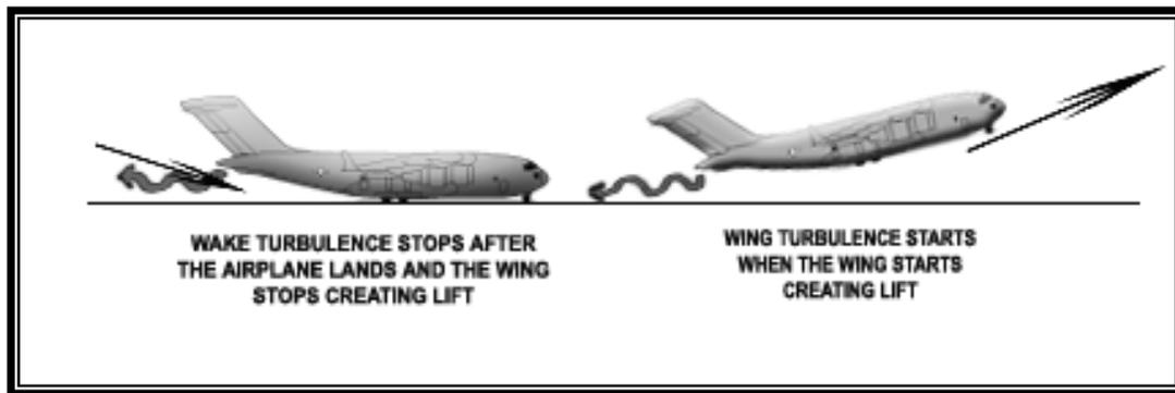
Crosswind blows wake turbulence from upwind runway into the approach path of the parallel runway. Smaller planes should cross above the possible area of turbulence and land well beyond the threshold.
